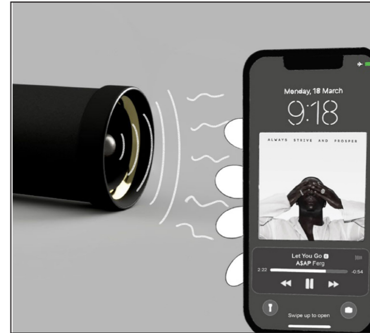
3. The user uses their device to connect to the speaker through bluetooth and is able to play music from their phone and adjust the settings of it.
